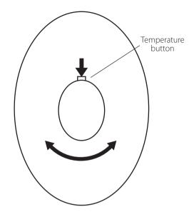
Turn the handle clockwise to increase the temperature and anti-clockwise to decrease the temperature.
