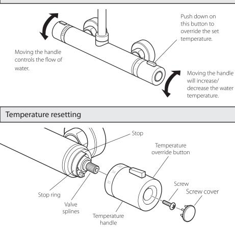
The valve has been factory set under balance pressures and hot water supply at 65° C. When your specific operating conditions are significantly different from the above, the temperature of the water may vary from the setting.
