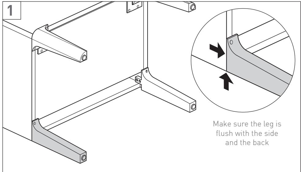
Line up the rear legs so they are flush with the sides and the back of the unit.
