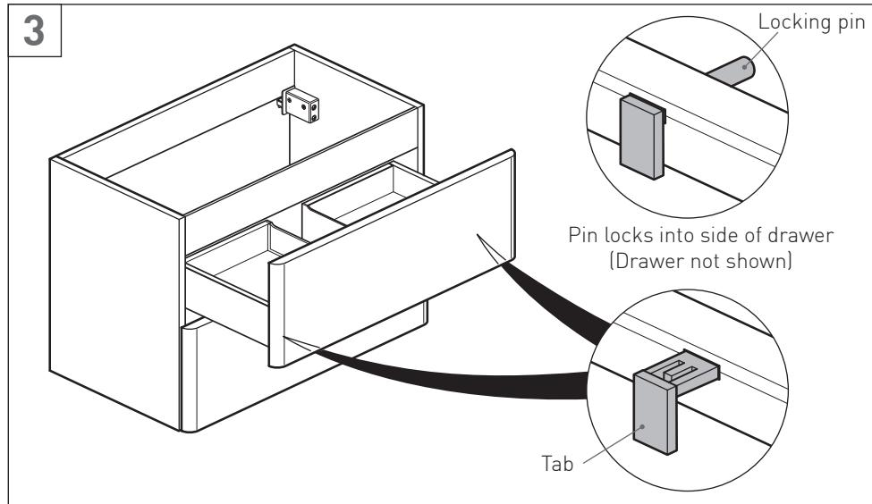
Remove the drawers prior to fitting the legs. Pull out a drawer so it's fully extended. On the underside of the runners, push each tab towards the centre of the unit until you hear a click.
