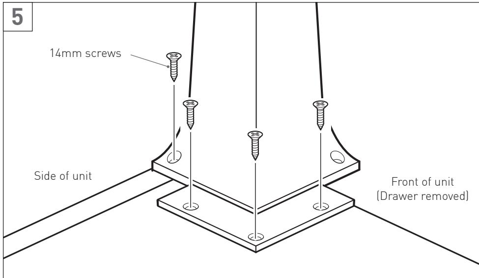
Line each bracket up to the marked points and screw in using four 14mm screws provided. Repeat for the other leg. Continue to page 9 if you are also installing the rear legs, otherwise proceed to the vanity installation guide.
