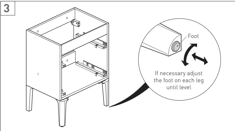
Place the unit into the desired location. If required, the unit can be leveled using the adjustable feet on the bottom of each of the four legs.
