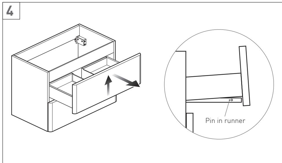
Gently lift the drawer forward to disengage it from the runner and remove from the cabinet. Repeat for the other drawer.
