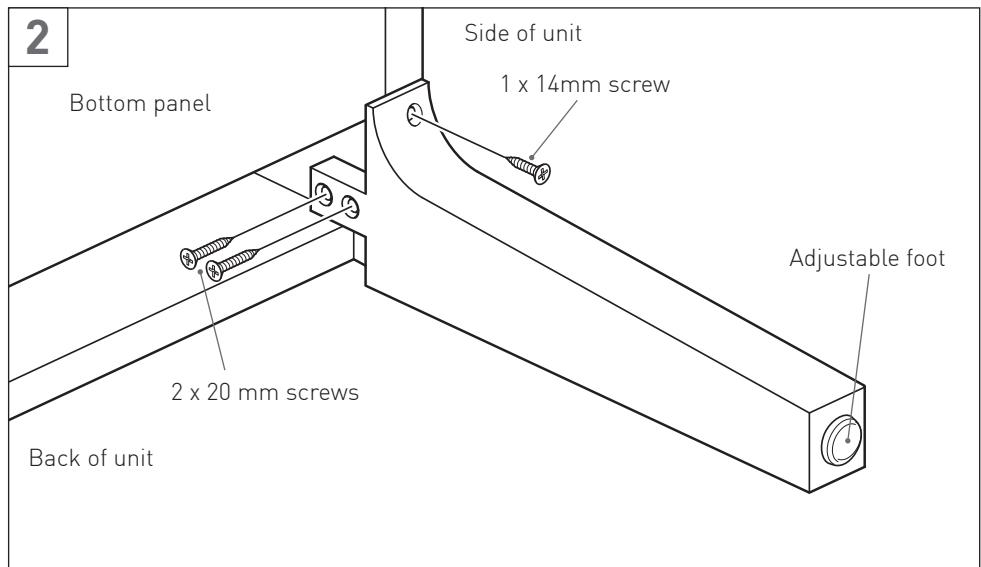
Attach the leg to the unit using the screws provided. The short 14mm screw is used at the front and the two longer 20 mm screws at the side.
