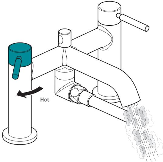
Turning the hot handle to the left will increase the flow of hot water.
