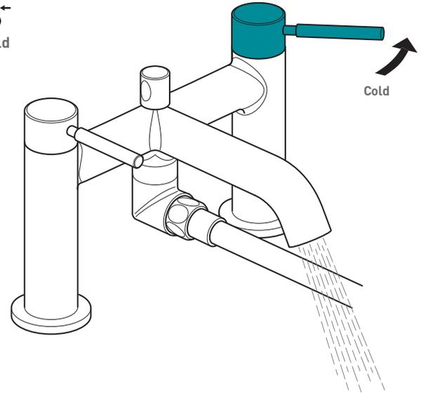
Turning the cold handle to the right will increase the flow of cold water.
