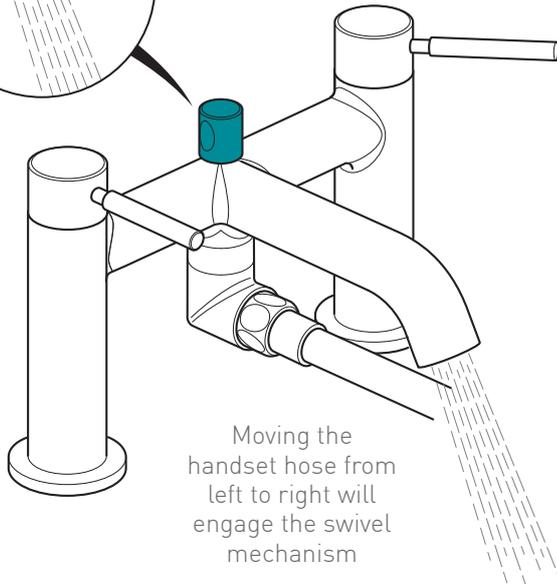
Moving the handset hose from left to right will engage the swivel mechanism
