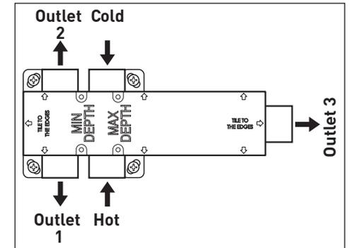
Finish the wall by tiling up to the mortar guard, keep the final finished wall surface between the min and max marks.
