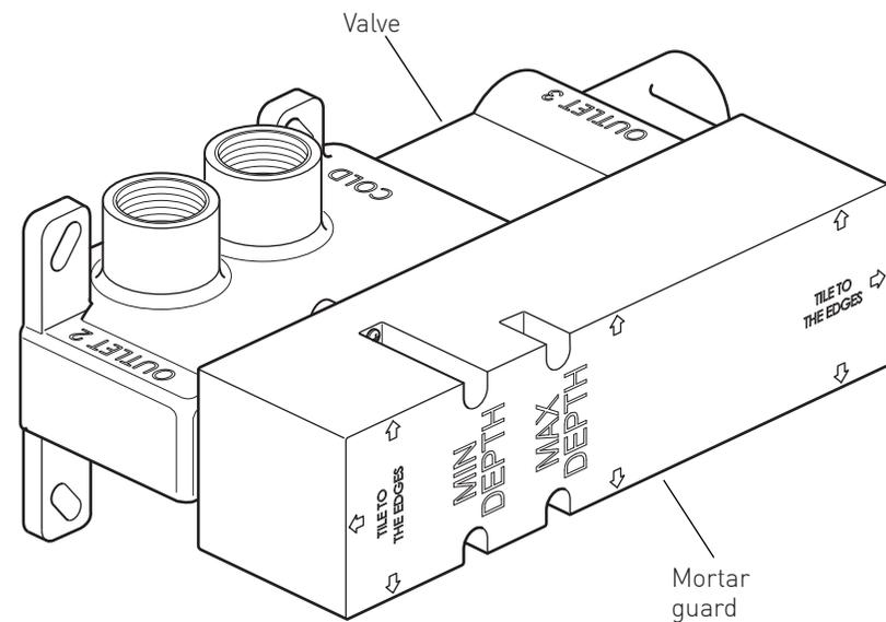
Flush pipe work thoroughly before fitting the valve.
