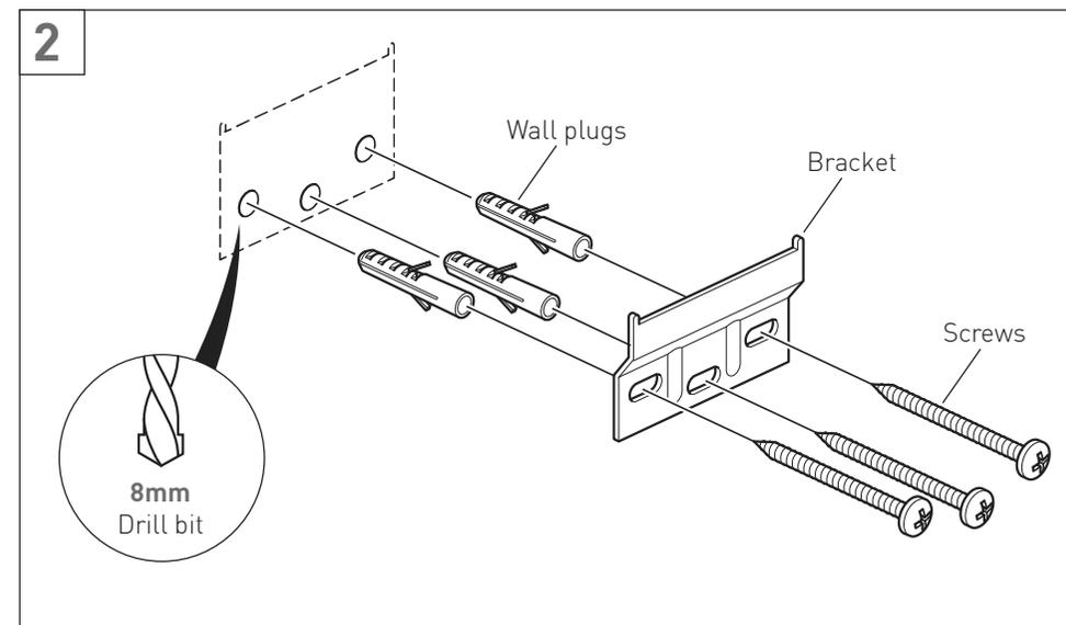
Drill  $\varnothing$  8mm holes, insert the wall plugs and screw on the brackets. **NOTE:** If the vanity unit and/or basin are not fitted level this may prevent the basin from draining correctly.
