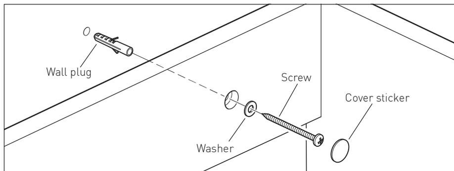
Solid Walls - Drill Ø 8mm holes into the wall through the holes in the bottom brace, insert a wall plug, washer and screw through each hole. Place the adhesive sticker over the hole.
