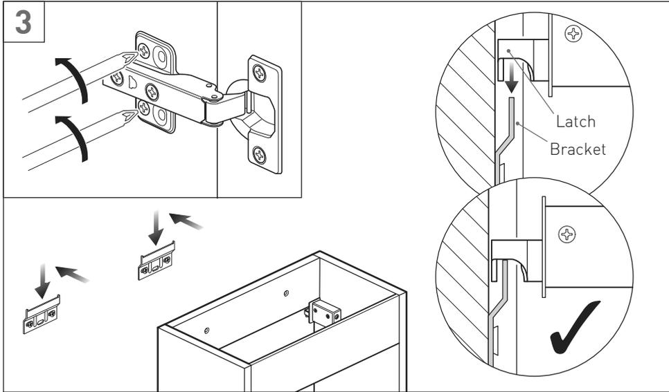
Remove the door of the vanity by unscrewing the hinges. With two people lift the unit over and onto the brackets, make sure that both latches are over the brackets before releasing the unit.
