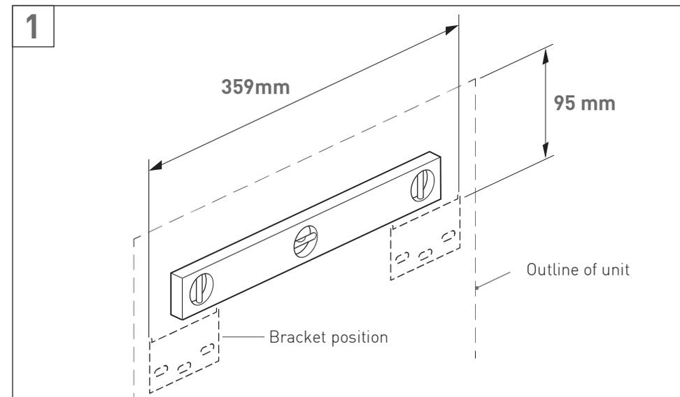
Decide on the position and height of the unit. The recommended basin height is between 800 and 850mm from floor to top of basin. Mark the bracket fixing holes onto the wall. **NOTE:** The dimensions are for the maximum width over the brackets.
