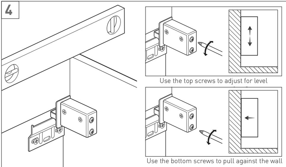
Check the unit is level. If leveling is required, use the top screw on both sides to lower or lift the unit. Once level, use the bottom screws on the hangers to clamp the unit to the wall.
