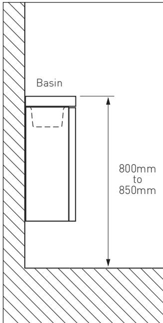
**For installations onto non solid walls, consult the diagram below.**
