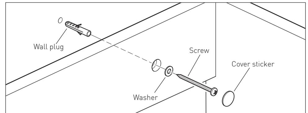
**Solid Walls** - Drill  $\varnothing$  8mm holes into the wall through the holes in the braces, insert a wall plug, washer and screw through each hole. Place the adhesive sticker over the hole.
