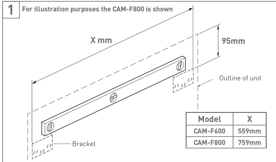
Decide on the position and height of the unit. The recommended basin height is between 800 and 900mm from floor to top of basin. Mark the bracket fixing holes onto the wall. **NOTE:** The dimensions are for the maximum width over the brackets.
