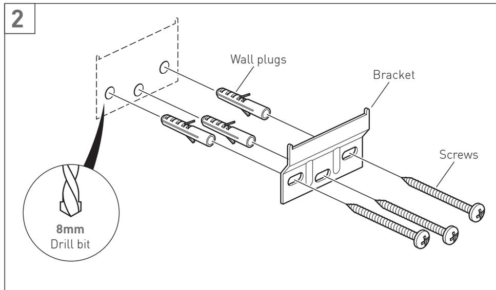
Drill  $\varnothing$  8mm holes, insert the wall plugs and screw on the brackets.
