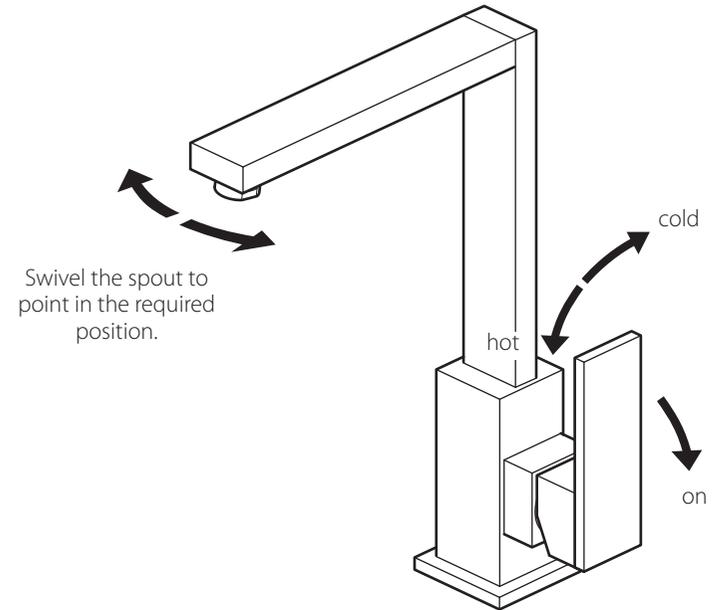
Moving the mixer lever outwards will increase the flow of water.
