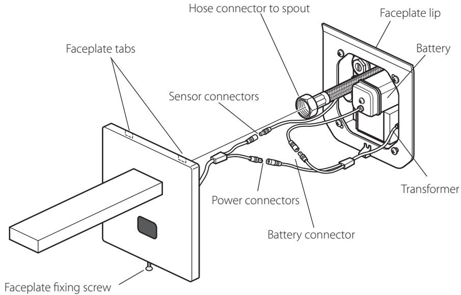
Connect the flexible hose coming from the unit onto the spout, making sure that the rubber washer is in place.
