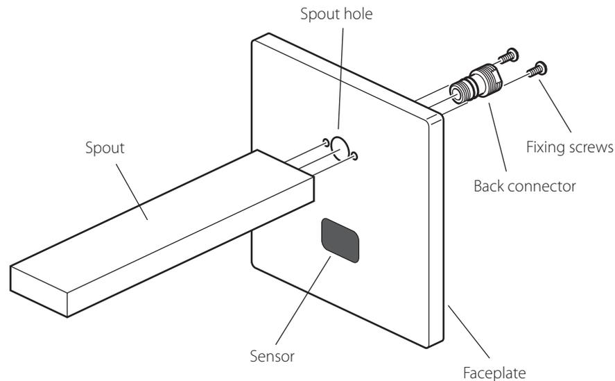
For ease of installation the faceplate and battery can be disconnected from the unit at the connectors.
