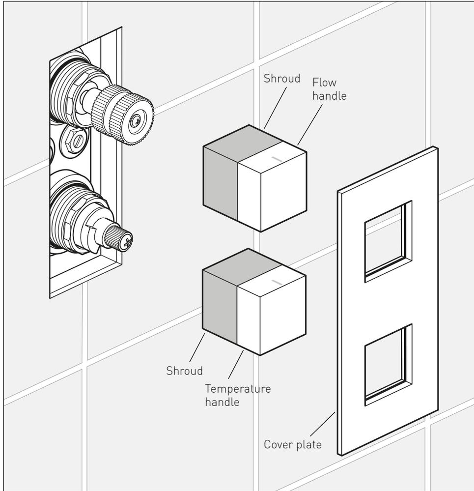
Screw the shroud assembly to the valve whilst holding the handle. Ensure the temperature handle is correctly located with the handle mark at 12 o'clock.
