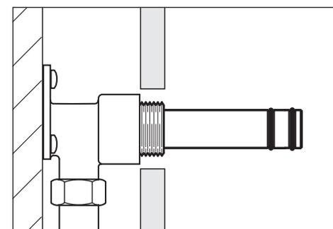
The connector should be flush with the wall. Remove the connector.
