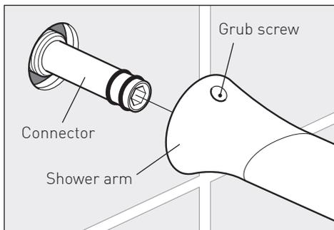
Tighten the grub screw using the hex key.
