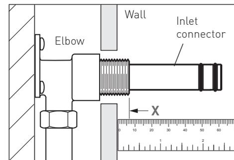
Remove the connector from the elbow. If necessary carefully cut the bottom of the connector by this measurement (**Xmm**) Remove any burrs.
