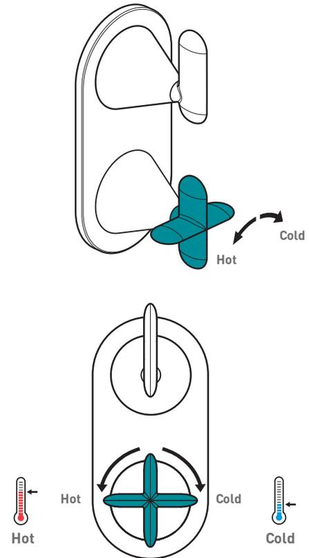
Turning the temperature control handle in the direction of the arrows increases/decreases the temperature
