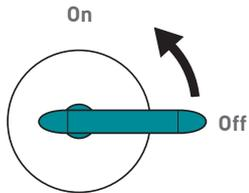
Turning the handle 90° anti-clockwise will progressively increase the flow of water to outlet 2.
