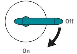
Turning the handle 90° clockwise will progressively increase the flow of water to outlet 1
