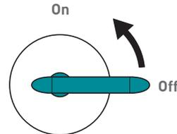
Turning the handle 90° anti-clockwise will progressively increase the flow of water to outlet 2.
