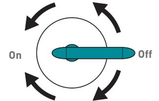
Turning the handle 180° will run both outlets simultaneously.
