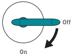
Turning the handle 90° clockwise will progressively increase the flow of water to outlet 1.
