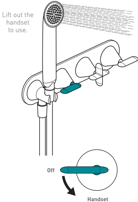
Turning the handle 90° anti-clockwise will progressively increase the flow of water to the handset
