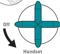
Turning the handle 90° anti-clockwise will progressively increase the flow of water to the handset (Outlet 2).
