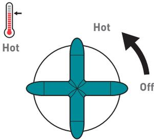
Turning the handle 90° anti-clockwise will increase the temperature.
