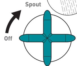
Turning the handle 90° clockwise will progressively increase the flow of water to the spout (Outlet 1)
