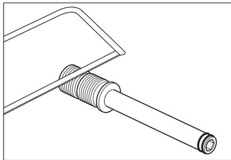
Check the spigot by screwing into the elbow, the inside of flange should be flush with the outside of the wall.
