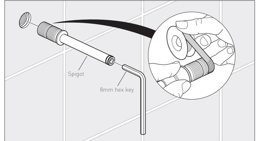
Using PTFE tape on the thread, screw the spigot into the wall and tighten using a 8mm hex key (not supplied).
