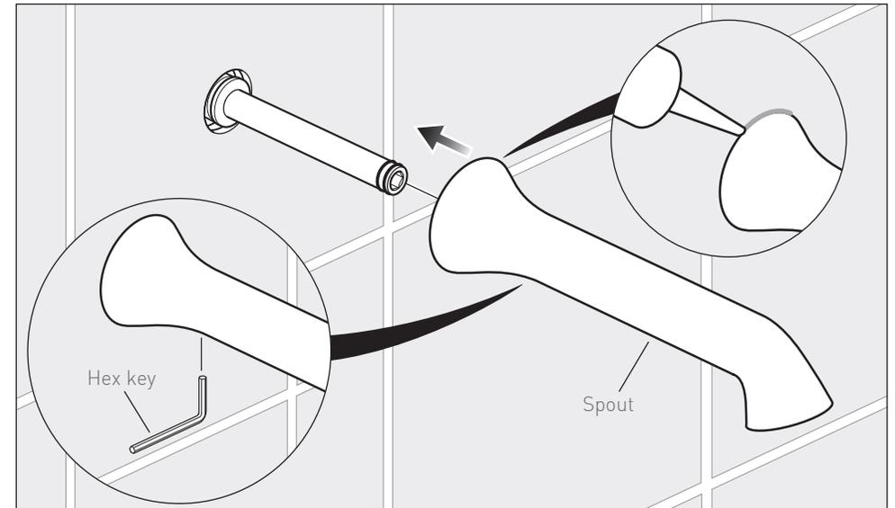
Carefully push the spout onto the spigot being careful not to damage the O-rings. Make sure that the spout is vertical and secure using the supplied grub screw on the underside of the spout. Apply a thin bead of silicone around the outside of the spout to seal against the tiles.
