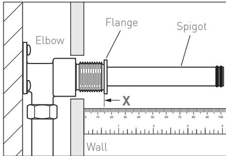
Screw the spigot into the connector/elbow. Take the measurement from the finished wall surface to the inside of the flange (X see right).
