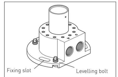
Connect the hot and cold supplies to the base. The hot should be fixed to the outlet marked **H** and the cold fixed to **C**.
