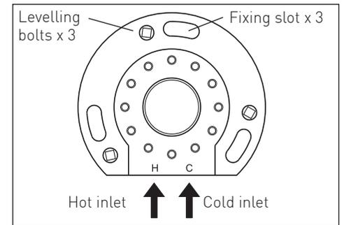
Position the base in the desired location, mark the 3 fixing holes. Remove the base and drill the 3 x holes to the required diameter and depth to suit your fixings.
