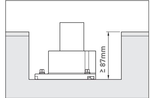
There are 3 fixing positions and 3 levelling bolts.
