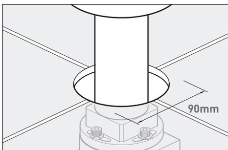
Slide the shroud down until it makes connect with the floor.
