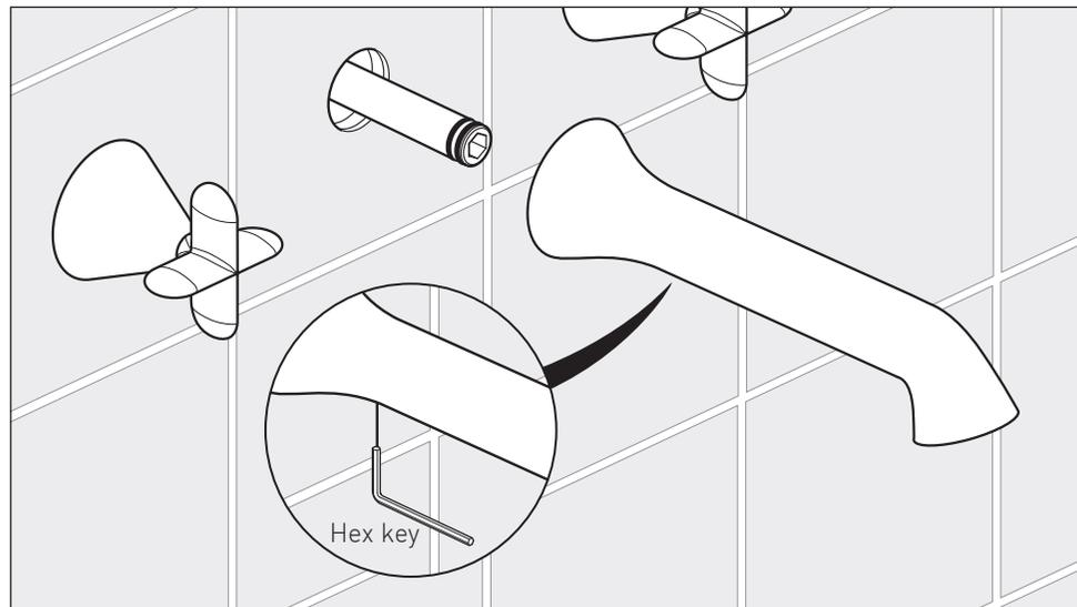
Carefully slide the spout over the O-rings and onto the spigot, make sure the spout is pointing downwards. Using the supplied hex key secure in position using the grub screw on the underside.
