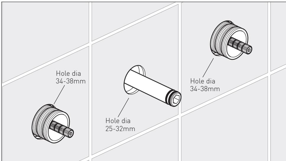
Finish the wall, tiles etc. Leaving spacing (between min and max hole diameters) around the three housings.
