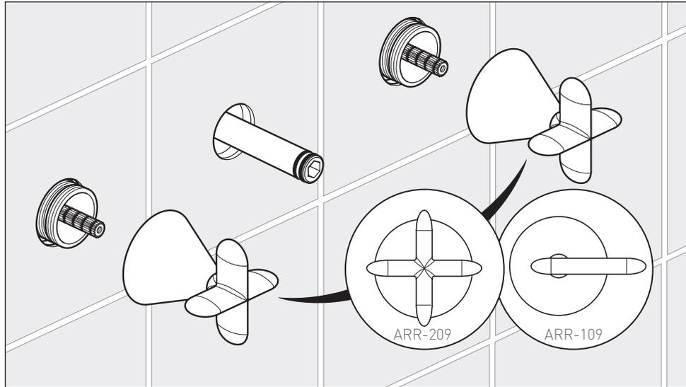
Carefully slide the handles onto the spline of the valve. While holding the handle in the cross position (levers vertical/horizontal) screw the shroud until touches the wall. For the ARR-109 the levers should be in the horizontal position.
