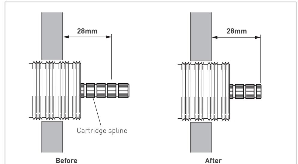
The cartridge spline will need to be cut down to 28mm from the finished wall. Mark 28mm from the finished wall and carefully cut using a hacksaw, remove any burrs.
