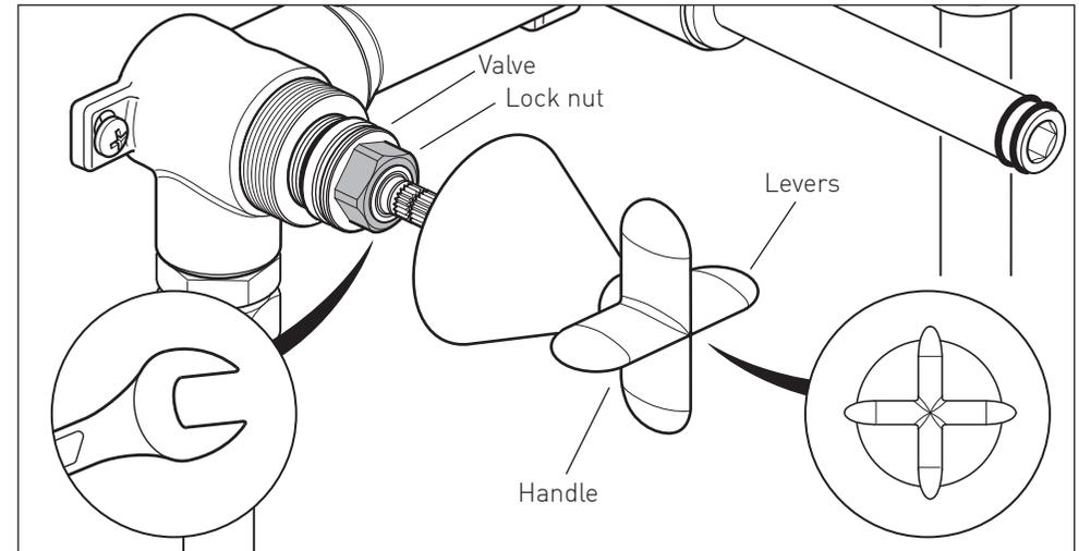
1. Unscrew the lock nut, remove it from the valve and place to one side. Then loosen the valve from the body, but do not remove.
