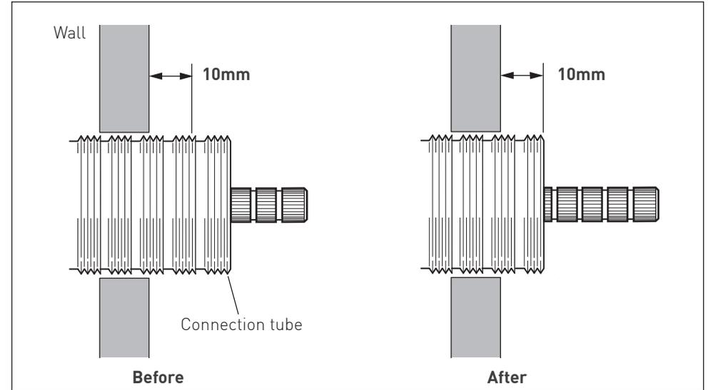
The threaded connection tube will need to be cut down to 10mm from the final wall surface. Mark 10mm from the wall and carefully cut using a hacksaw, remove any burrs.
