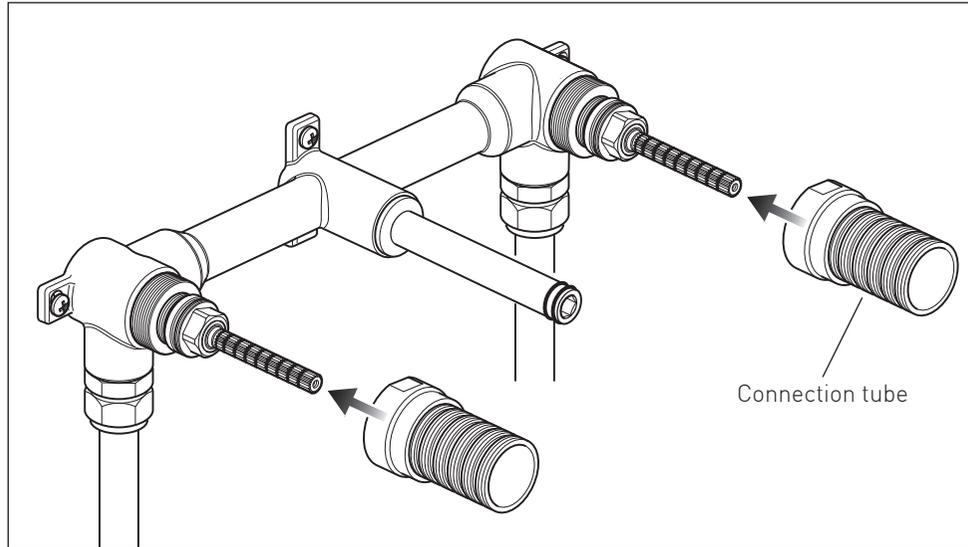
Screw the two threaded connection tubes back onto the valve. Tighten using a spanner on the spanner flats.
