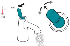
Rotating the handle to the left changes flow and temperature simultaneously.
