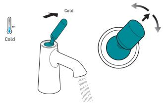
Rotating the handle to the right changes flow and temperature simultaneously.
