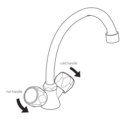
Turn the handles anti-clockwise to increase the flow of water and clockwise to decrease the flow.
