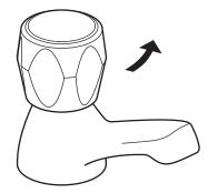
Cold tap - turning the control handle anti-clockwise will increase the flow of water.
