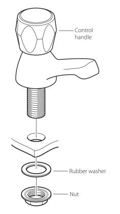
Before installing your new tap, flush through the pipework to ensure removal of debris, turn off the water supply.
