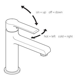
Moving the mixer lever upwards/downwards will increase/decrease the flow of water. Moving the mixer lever from right to left will increase the water temperature.
