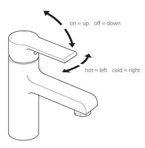
Moving the mixer lever upwards/downwards will increase/decrease the flow of water. Moving the mixer lever from right to left will increase the water temperature.
