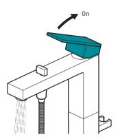
Moving the mixer lever upwards/downwards will increase/ decrease the flow of water.
