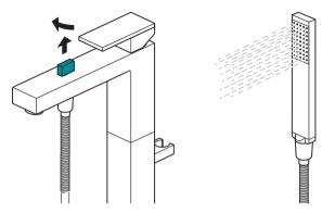
Pull up the diverter handle and turn clockwise to lock into position.
