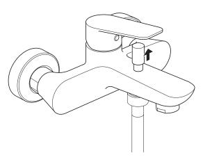
Pull the shower control knob up to turn on the shower, turn to lock in position. Turn back to release and turn off the shower.
