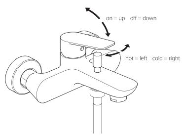
Moving the mixer lever upwards/downwards will increase/decrease the flow of water. Moving the mixer lever from right to left will increase the water temperature.
