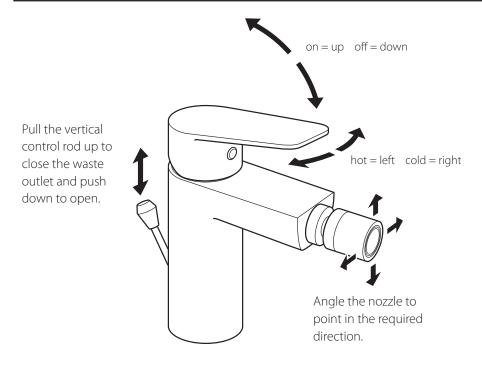
Moving the mixer lever upwards/downwards will increase/decrease the flow of water. Moving the mixer lever from right to left will increase the water temperature.
