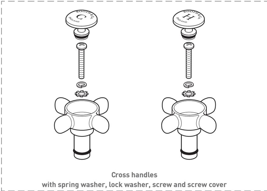
Cross handles with spring washer, lock washer, screw and screw cover
