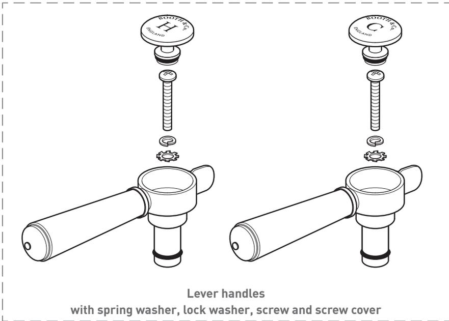
Lever handles with spring washer, lock washer, screw and screw cover
