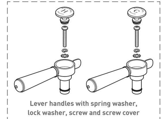
Lever handles with spring washer, lock washer, screw and screw cover
