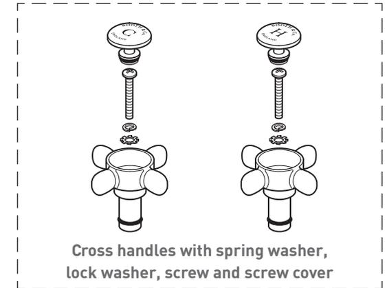
Cross handles with spring washer, lock washer, screw and screw cover
