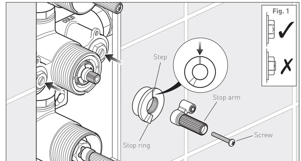
Push the stop ring onto the splines of the cartridge, making sure that the step on the stop ring is at 12 o'clock. Slide the stop arm on and secure in position with the screw.
