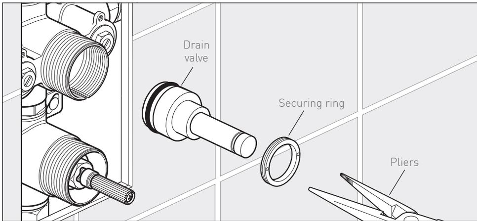
Remove the speedfit connector. Using a pair of long-nosed pliers unscrew the securing ring and remove. Pull the drain valve out from the body
