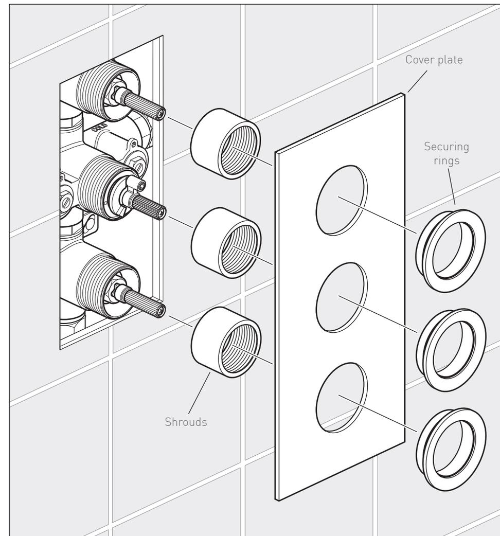
Screw shrouds on ensuring they sit proud of the finished wall. The shrouds can be turned/adjusted to achieve this.
