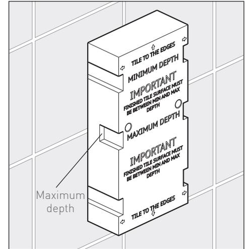
Finish the wall by tiling up to the mortar guard, keep the final finished wall surface between the min and max marks. Unscrew the 2 mortar guard screws and remove from the wall.
