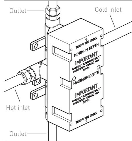
Use the supplied adapters if required. Connect hot supply to the left inlet of the valve and cold supply to the right inlet. Connect the top and bottom outlets to the desired channels.
