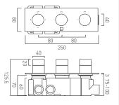
knurled Accents Tablet 3 outlet 3 handle horizontal concealed thermostatic shower valve with all-flow function thermostatic cartridge V-704-34S diverter cartridge FL-802-33/2MX flow cartridge TAB-002A-3/4 2 x 3/4" female inlets 2 x 3/4" female outlets includes 3/4" - 1/2" adaptors tile-to mortar guard included min-max wall mount 75-100mm optimum installation depth 87mm minimum operating pressure 0.2 bar LP (shower) 1.0 bar MP (bath)
