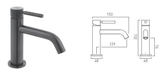
Knurled Accents slimline mono basin mixer single lever deck mounted smooth bodied without universal basin waste with water flow aerator ceramic cartridge C-010-N25 2 x 1/2" 400mm flexipipe connections deck mount drill hole diameter 35mm minimum operating pressure 1.0 bar MP
