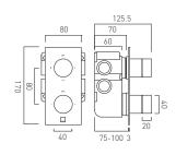
knurled Accents Tablet 2 outlet 2 handle vertical concealed thermostatic shower valve with all-flow function thermostatic cartridge V-704-34S diverter cartridge FL-802-33/2MX 2 x 3/4" female inlets 2 x 3/4" female outlets includes 3/4" - 1/2" adaptors tile-to mortar guard included min-max wall mount 75-100mm optimum installation depth 87mm minimum operating pressure 0.2 bar LP (shower) 1.0 bar MP (bath)
