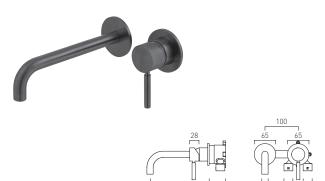
knurled Accents slimline 2 hole basin mixer single lever, wall mounted with water flow aerator ceramic cartridge CAR-K35B 2 x 1/2" inlets min-max wall mount 55-72mm tile-to mortar guard included wall mount drill hole diameters: spout 40-48mm handle 45-48mm minimum operating pressure 0.2 bar LP
