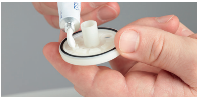
Position the hinges and then glue in place with the high strength adhesive supplied.
