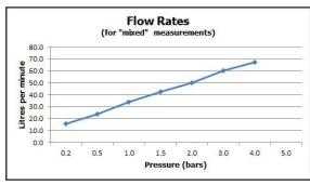
'mixed measurements' refers to equal hot and cold water supply flow rate for unregulated flow unless flow regulator fitted as standard  $\,$
