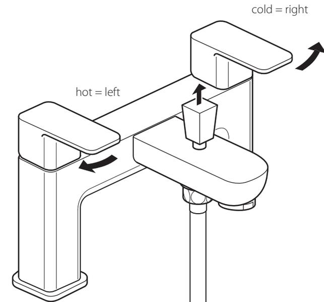
Moving the levers in the direction of the arrows will increase the flow of water. Pull the shower control knob up to turn on the shower, turn to lock in position. Turn clockwise again to release the diverter and go back to the primary outlet.
