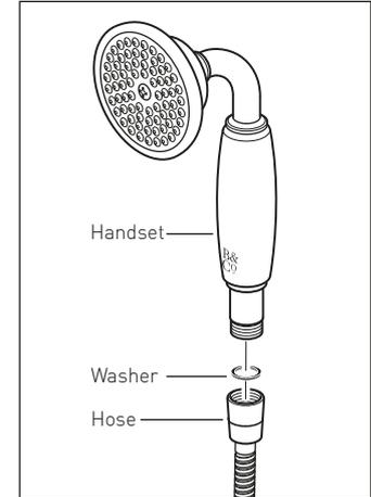
Place the second rubber washer into the nut end of the hose and attach it to the valve/outlet.
