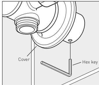
Slide the cover along until it makes contact with the wall.
