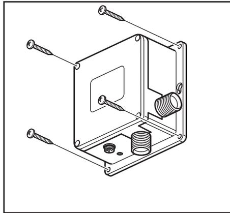
Make sure that the rubber washers are in place in the flexible pipes. Connect the flexible pipe from the tap to the bottom outlet marked 'Outlet'. Connect the other flexible pipe to the side connection marked 'Inlet'.
