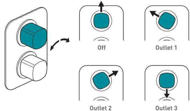
Turning the flow control handle to the required position increases the flow of water
