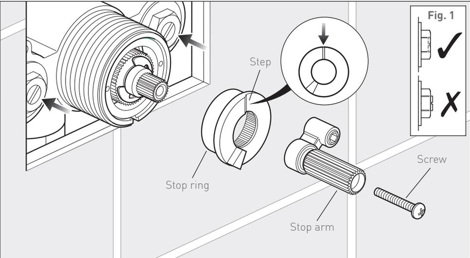
Push the stop ring onto the splines of the cartridge, making sure that the step on the stop ring is at 12 o'clock. Slide the stop arm on and secure in position with the screw. Open both non return valves.
