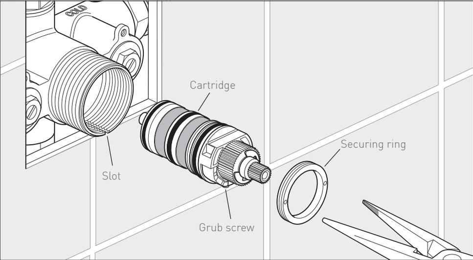
Push the cartridge into the body, align the grub screw with the slot and continue to push the cartridge all the way in.
