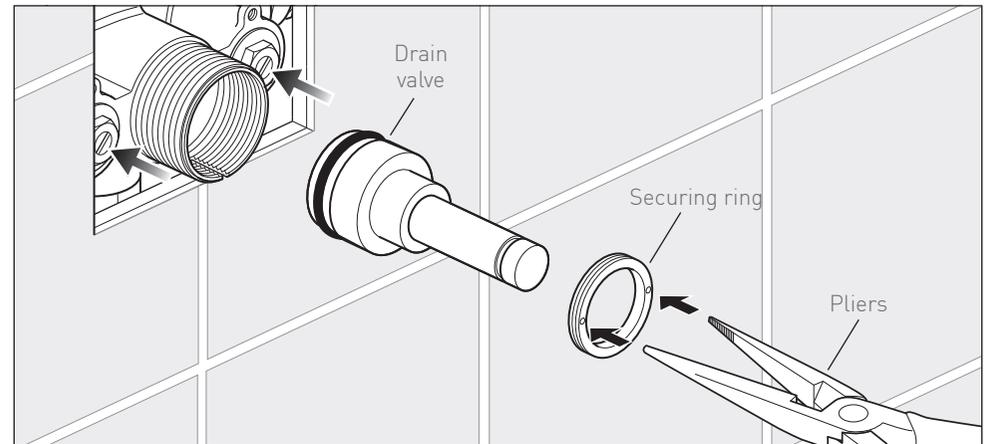
Close both non return valves. Remove the speedfit connector. Using a pair of long-nosed pliers unscrew the securing ring and remove. Pull the drain valve out from the body
