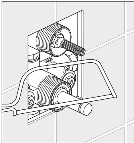
**Important:** ensure the hot and cold water supplies have been isolated. Using a suitable tool, cut the end off the drain through the easy cut section.
