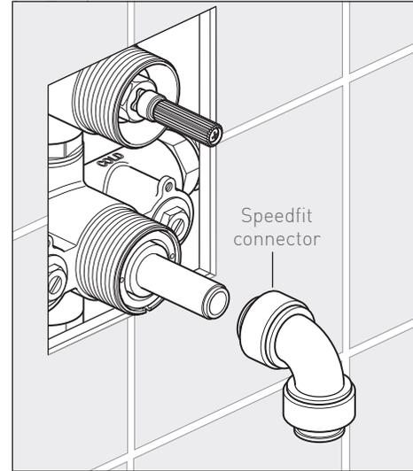
We recommend to push a speedfit connector (not supplied) over the drain, and place a bucket underneath. If a speedfit connector is not being used, carefully hold a bucket underneath the drain valve.
