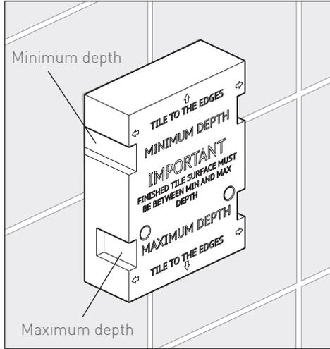
Finish the wall by tiling up to the mortar guard, keep the final finished wall surface between the min and max marks. Unscrew the 2 mortar guard screws and remove from the wall.
