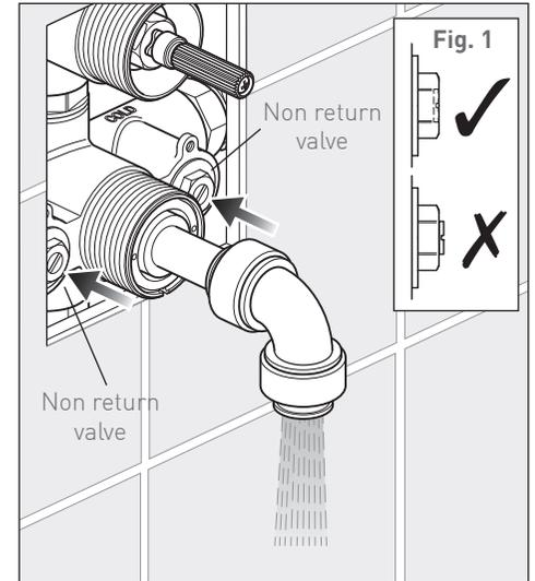
Turn on at the mains, open both non return valves and allow the debris and water to drain. When loosening the non return valve do not unscrew further than the face of the nut (see Fig. 1). After approximately two minutes of flushing the pipe work and product close both non return valves. Do not overtighten.
