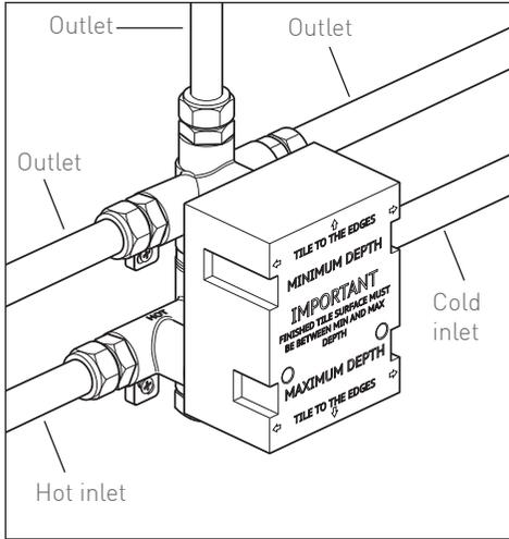
Connect hot supply to the lower left inlet of the valve and cold supply to the lower right inlet. Connect the open outlets to desired channels.
