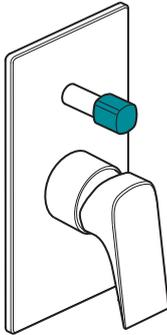
Pull the diverter handle and turn clockwise to lock into position. Turn clockwise again to release the diverter and go back to the primary outlet.
