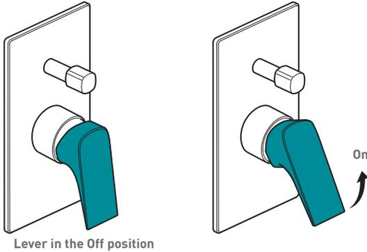
Pulling the mixer lever outwards will increase the flow of water.
