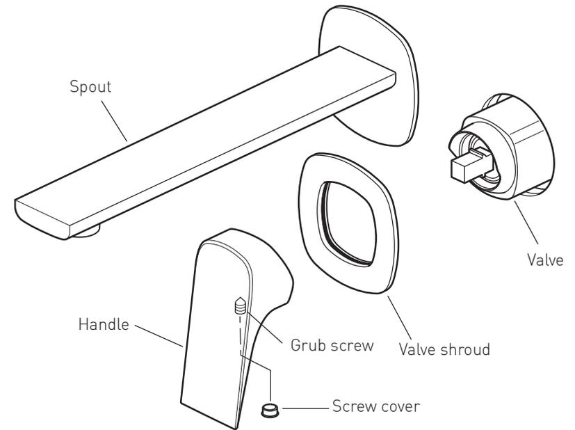
Make sure that the O-ring is in place in the back of the shroud. Slide the shroud carefully over the valve being careful not to dislodge the seal on the inside. Carefully slide the control handle onto the valve. Secure in position with the grub screw within the handle using the hexagonal key supplied. Push on the screw cover.
