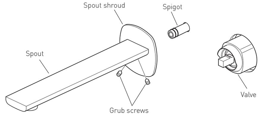
Make sure that the O-ring is in place in the back of the shroud. Slide the spout over the spigot until the shroud is in contact with the wall. Secure the spout using the two grub screws on the underside, tighten with the supplied hex key.
