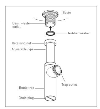
The outlet pipe can be cut to the required length. Ensure all calculations are correct before cutting, remove any burrs before assembly.
