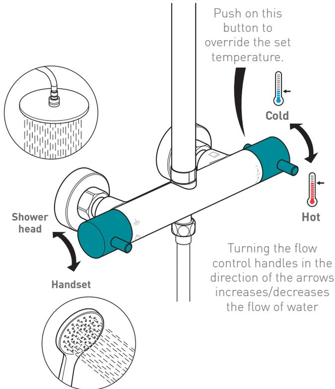
Turning the handle in the direction of the arrows diverts the flow of water between the shower head and handset
