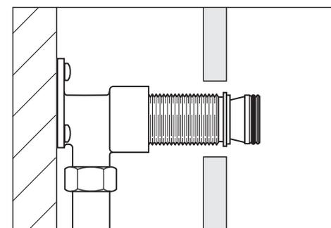
The distance between the wall and the end of the connector should be 13.5mm. Remove the connector.
