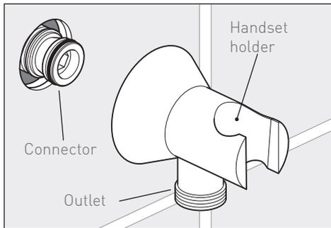
Tighten the grub screw on the underside using a hex key. Apply a thin bead of silicone around the outside of the outlet to seal against the tiles.
