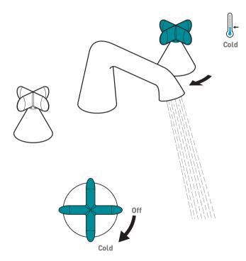
Turning the hot handle anti-clockwise will increase the flow of hot water.
