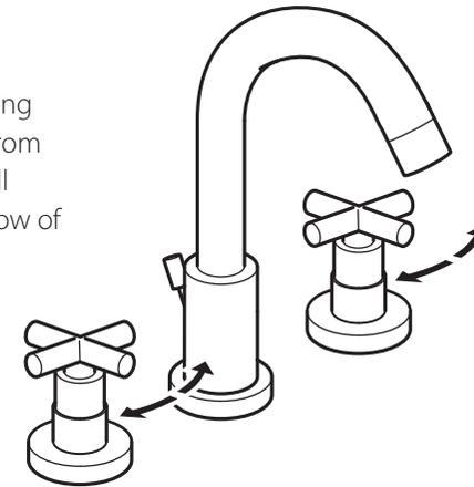
Cold tap - moving the tap lever from left to right will increase the flow of water.
