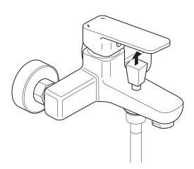
Pull the shower control knob up to turn on the shower, turn to lock in position. Turn back to release and turn off the shower.
