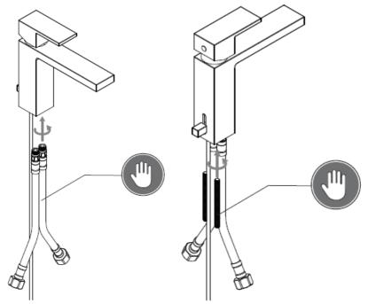
Place the 2 threaded rods and 2 flexible pipes into the body of the mixer.
