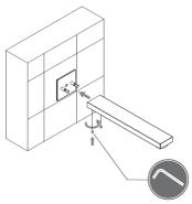
Slide the spout over the two pins emerging from the plaque assembly. then screw back in the previously removed screw on the bottom of the spout and fix them (hex key 2mm). Be careful that the O-ring on the spout remains in place during the operation.
