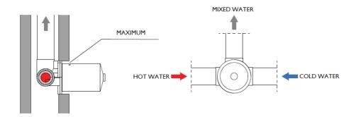
Install the mixer housing at a depth so that the finished surface is no further than the maximum distance marking shown in the diagram.
