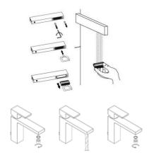
Periodically the aerator will need to be cleaned, simply remove the 2 retaining screws. Or unscrew the aerator
