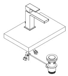
Install the flexible pipes, Open the water supplies and test for leaks on the connections.
