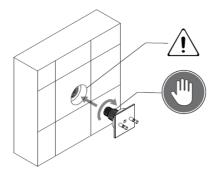
Then screw the insert into the wall water outlet fixing it by hand. making sure there is enough space into the wall to insert the brass collar.
