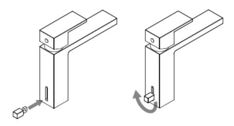
Insert the pop-up knob into the back-side of the mixer body, then rotate it  $90^{\circ}$  as shown above.
