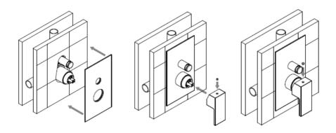
Once the surrounding finishes have been applied (Tiles/Marble etc.) remove the protection covers. Fit the face plate onto the mixer body, it is advised to use a small amount of lubricant on the rubber seals. Slide the handle onto the cartridge pin and secure with the grub screw, then push on the cover cap.
