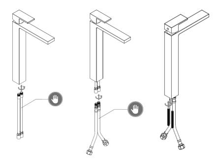
Place the 2 rigid pipes followed by the 2 threaded rods and 2 flexible pipes into the body of the mixer.
