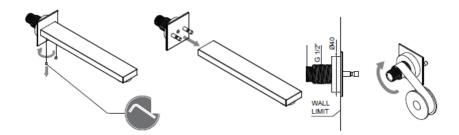
Remove the two screws under the spout (hex key 2mm). pull the spout in order to separate it from the plaque assembly. Wrap the threaded end of the plaque assembly using P.T.F.E thread seal tape or hemp.
