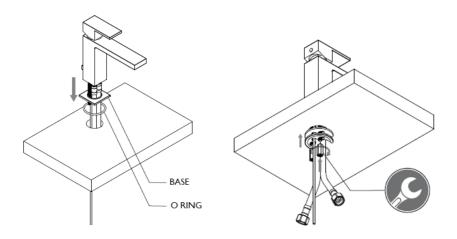
Install the 'O' ring and place the assembly through the basin / counter, From the underside, place the 'C' ring followed by the metal 'C' washer onto the threaded rods, then tighten to clamp the mixer to the basin / counter with the back nuts, being careful not to over tighten.
