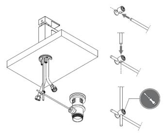
Install the waste ensuring that the foam washer is in between the waste and the basin on the top portion of the waste, the rubber washer is to be placed under the basin before the bottom part of the waste is connected and tightened up. Again take care not to over tighten.
