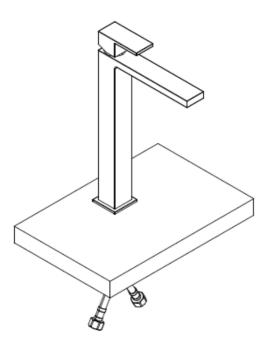
Install the flexible pipes, Open the water supplies and test for leaks on the connections.
