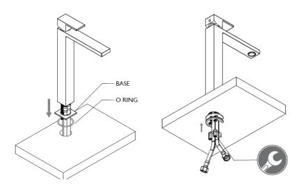
Install the base and 'O' ring and place the assembly through the basin / counter, From the underside, place the 'C' ring followed by the metal 'C' washer onto the threaded rods, then tighten to clamp the mixer to the basin / counter with the back nuts, being careful not to over tighten.
