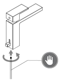
Whilst holding the pop-up knob in place, from underneath hand-tighten the pop up rod into the thread of the pop-up knob.
