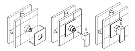
Once the surrounding finishes have been applied (Tiles/Marble etc.) remove the protection covers. Fit the face plate onto the mixer body, it is advised to use a small amount of lubricant on the rubber seals. Slide the handle onto the cartridge pin and secure with the grub screw, then push on the cover cap.
