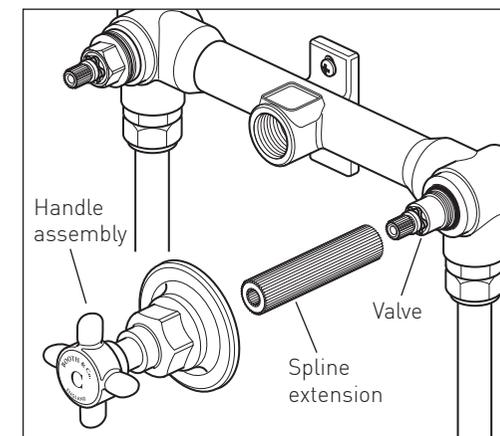
Using light force only turn the handle clockwise until you feel a noticeable resistance when the base of valve touches down on the body of the tap.
