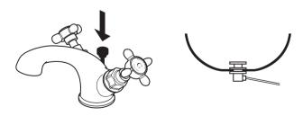
Push the waste control rod down to open the plug and empty the basin.
