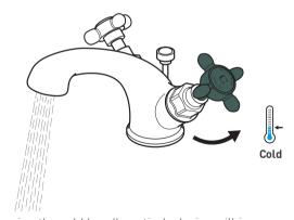
Turning the cold handle anti-clockwise will increase the flow of cold water.
