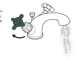
Turning the hot handle clockwise will increase the flow of hot water.
