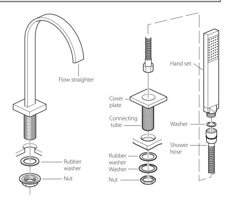
Ensure that the 'O' ring is in place in the underside of the cover plate. Position the spout in place , and from the underside slide on the rubber washer and then the nut. Tighten the nut to clamp on the spout.
