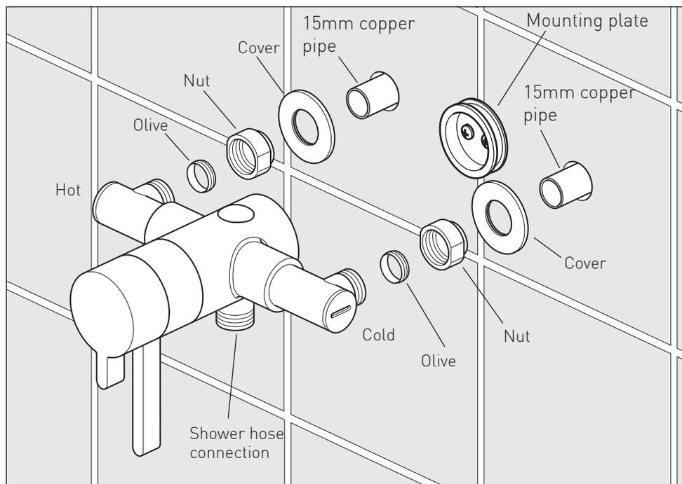
During and after installation protect the outer parts of the valve to avoid damage to plated surfaces.
