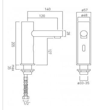
description: zoo infra-red mono basin mixer with rub clean aerator deck mounted mains or battery operated takes standard AA batteries ceramic cartridge IR-100/CONTROL finishes: chrome
